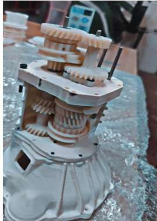
Fig. Assembly of 5 speed Gearbox
